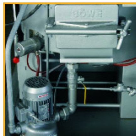
The automatic emission free still rake out system requires no manual intervention in normal operation
